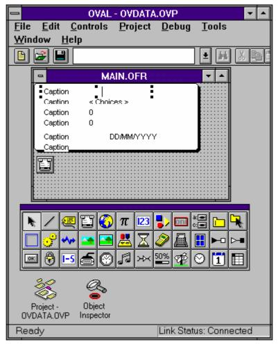
Examples controls are: text, menus, buttons, input fields, each control has information associated with it: its physical appearance, its current state, the things the user can do to it and with it (its events), and the code that determines what the application does in response to a given event.
