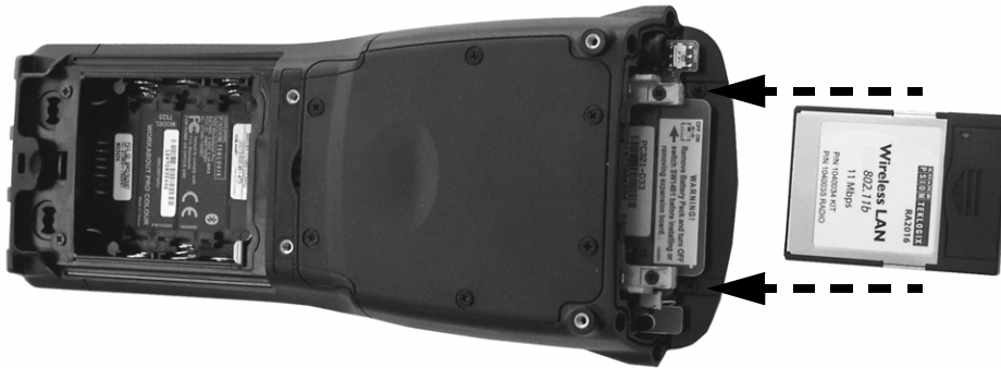
Figure 5.2 Inserting A CF Card
