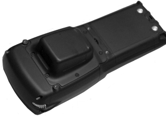
Figure 8.10 Scanner Module Installed In WORKABOUT PRO
