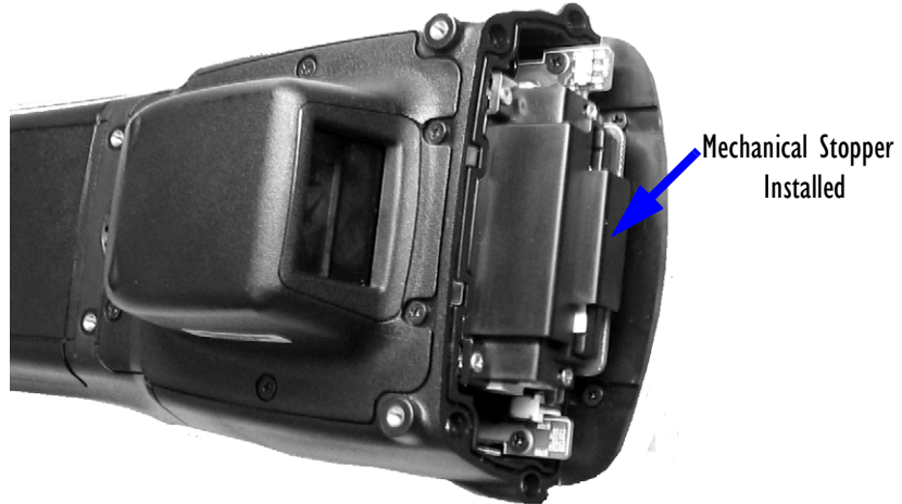
Figure 5.4 Mechanical Stopper Installed
