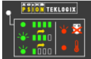
Figure 9.7 Battery Charge Status
