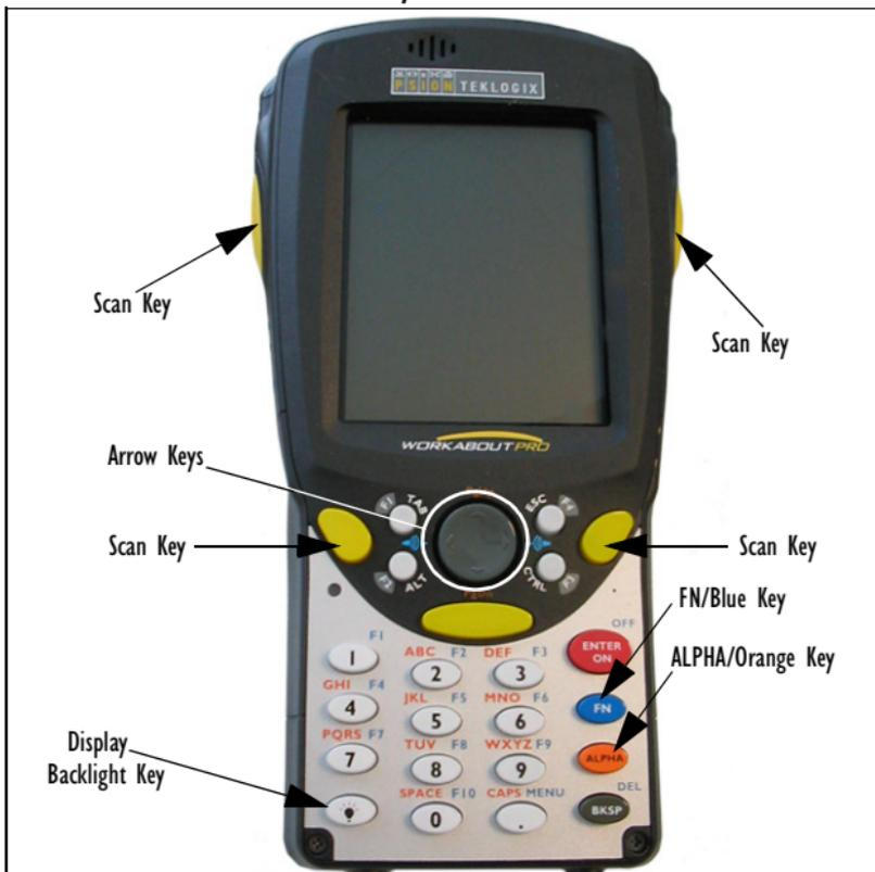
The keyboard is equipped with a set of standard keys along with an [ORANGE] and a [BLUE] modifier key to provide access to additional keys and system functions. These additional keys are colour coded in *orange* and *blue* print above the standard keys.
