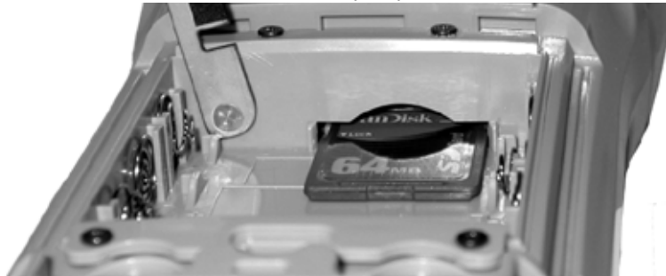
Figure 2.3 Location Of MMC/SD Card Slot
