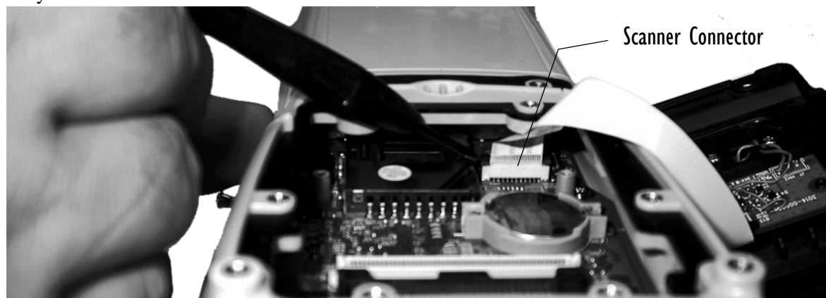
Figure 9.2 Location Of The Scanner Connector
