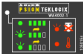
Figure 2.3 Battery Charge Status
